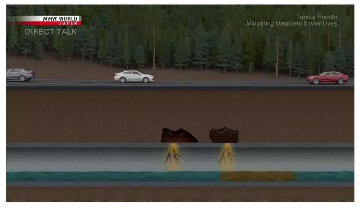
When an earthquake strikes, sewer pipes and other underground systems are damaged. When dirt or sand gets into the pipes, it can cause underground cavities to form.
